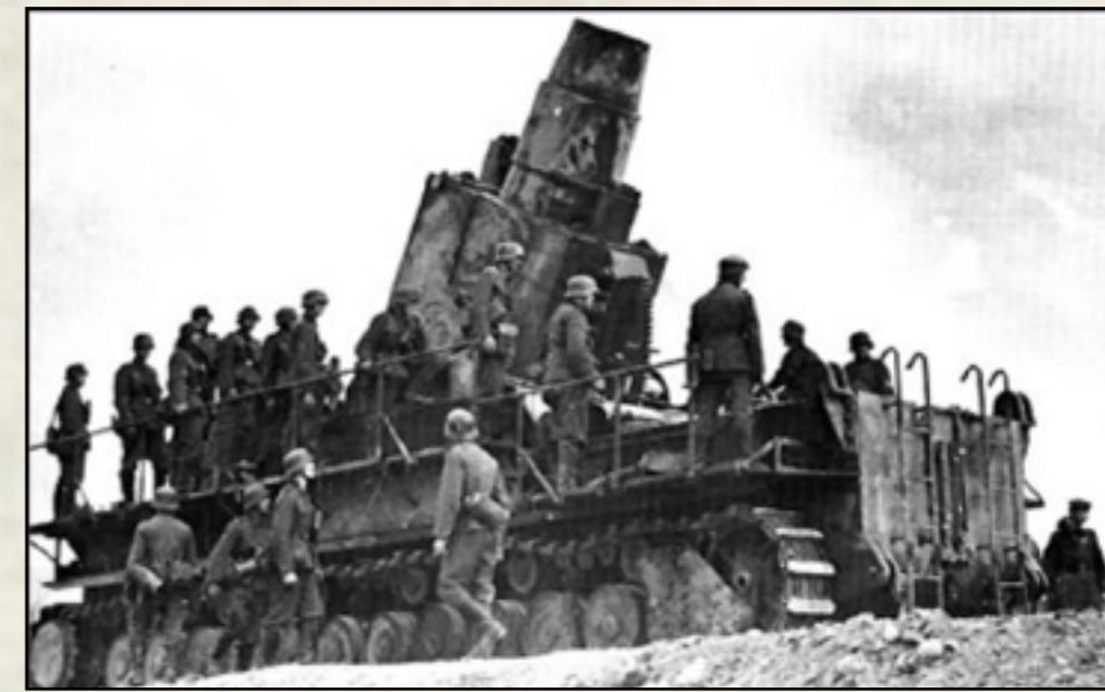
PACKING A PUNCH: The most powerful artillery gun created by any nation and used in WWII was named Karl by its designer General Karl Becker. Used mostly against the Russians, the huge gun could shoot a 2.5 ton shell over three miles. The shells were almost 61 cm wide and could go through three metres of concrete.
